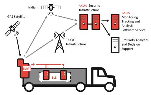
The AKUA SLE devices are attached to the cargo inside the container. They send data to the master device (SLM). The location of the container is monitored via GPS. Cargo data from the SLEs are transmitted via the master through the GPRS cellular data network or Iridium to the AKUA security infrastructure and then to the AKUA Monitoring, Tracking and Alerting Software Service or the user's proprietary application.
